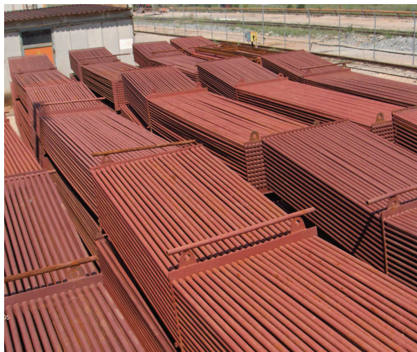
Figure 2. Overview of the heat pipes bundles before installation.
