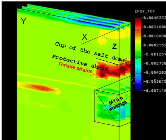
Fig. 14. Distribution of the strain  $\varepsilon_y$ , after 50 years in the roof shelf, in vertical cross-sections;  $X \in [1000, 1050, 1100 \text{ m}]$ ,  $\max \varepsilon_y \in [+4.6\%, +3.6\%, +2.9\%]$
