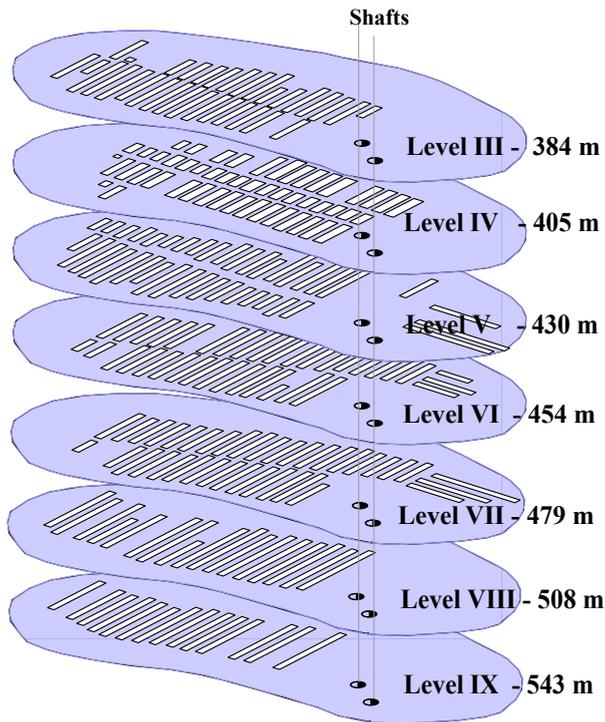
Fig. 1. The diagram of the distribution of rooms at Levels III-IX
