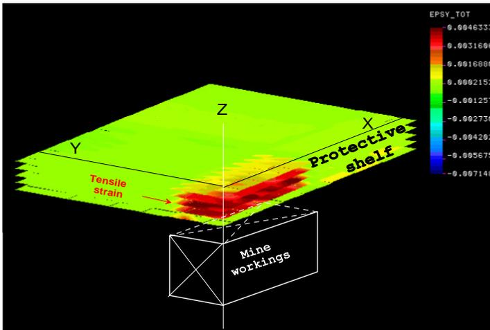
Fig. 15. Locations of the maximum horizontal strain  $\max \varepsilon_y$ , after 50 years, in horizontal cross-sections;  $Z \in [-220, -260 \text{ and } -300 \text{ m}]$ ,  $\text{Max}[\max \varepsilon_y(H)] = +4.64\%$
