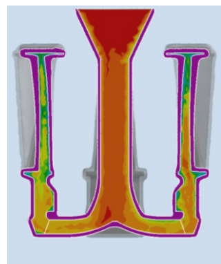
Fig. 6. An example of filling process of gating system with bottom filling (Step 2)
