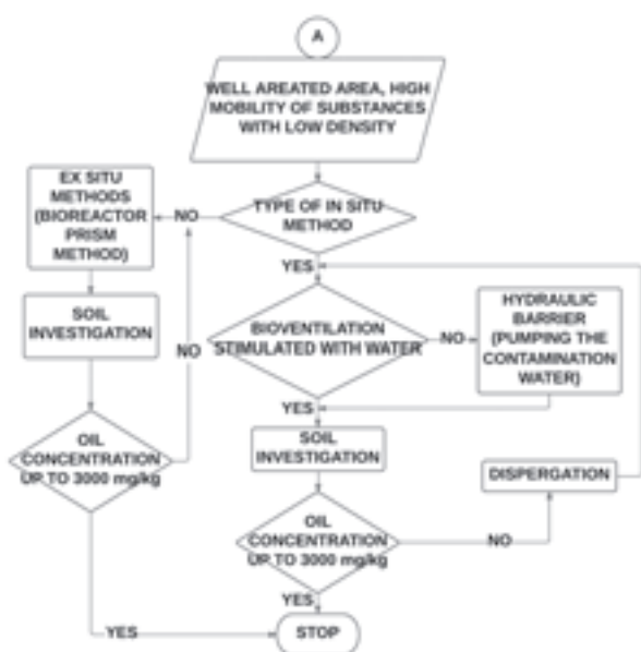
Fig. 2. Selection algorithm for remedial operations in case of well-aerated soil
