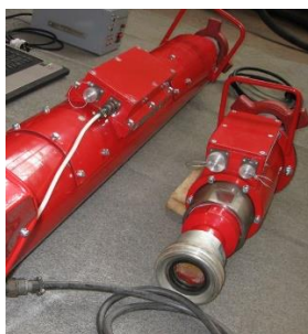
Fig. 12 Control station of technological operations SKTsS -01
