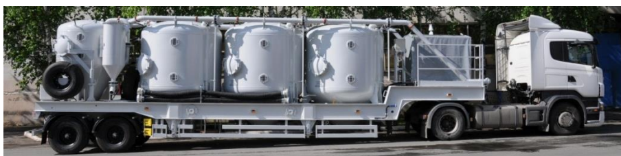
Fig. 10 Mobile cement bulk storage TsT-40
