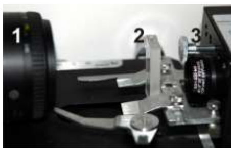
Fig. 3. The Shadow Sizing rig - the measurement stage, where: 1 - camera's lens' ring, 2 - the cuvette on the table, 3 - diffusion filter with the laser's optical system
