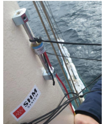
Fig. 3. STS Fryderyk Chopin side view with location of sensors in the first (circle) and the second (triangles) measurements series. Installation of vibrating wire strain gauges [12] [13].
