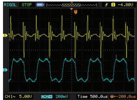
Fig. 10. Waveform of the input voltage ( U_{R0} )
