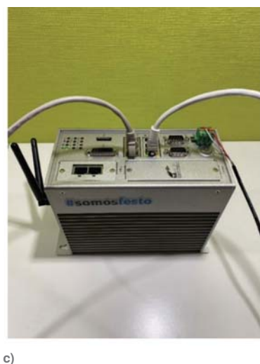
Fig. 6. Power supply and control devices for the test stand with EXPT tripod: a) CMMT-AS servo driver by FESTO AG & KG with connected: temperature sensors, brakes, motor phases and an encoder, b) KEBA AG robotic controller with a digital module and connected: I/O signals, servo drives (EtherCAT), Teach Pendant and IPC (Ethernet), c) industrial computer (IPC) with balenaOS operating system, optimized for running software packages (containers), including packages responsible for the operation of the Scraitec platform
