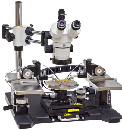
Fig. 1. MPS150 probe station by Form Factor company [2].
