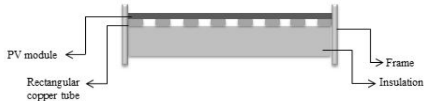
Fig. 1. Cross-section of the PV/T module [1]
