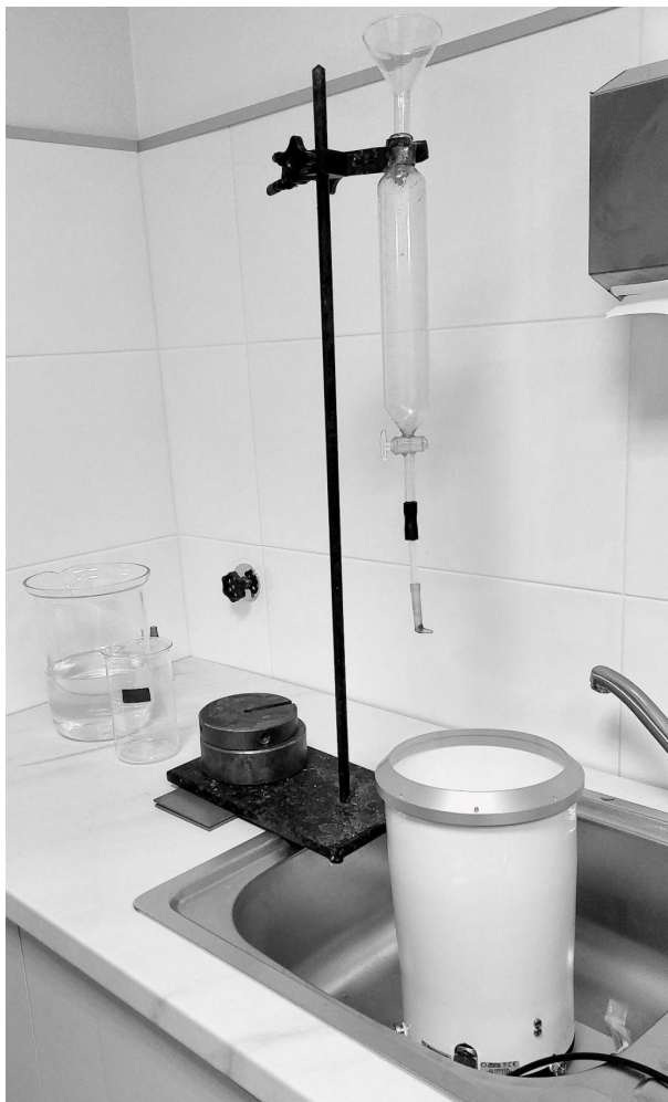
Fig. 6. Experiment stand B – rainfall simulated using dropper
