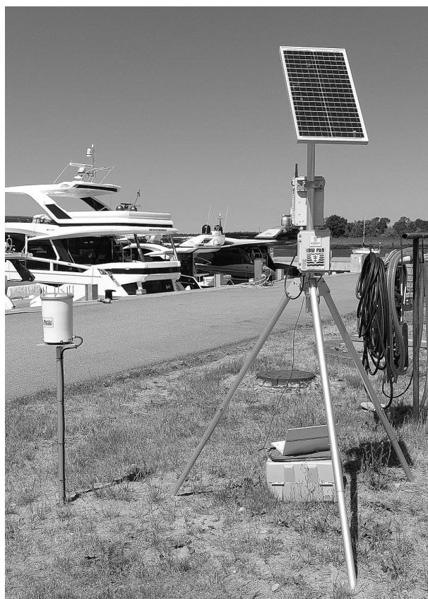
Fig. 1. Atmospheric precipitation station installed at Wiślinka
