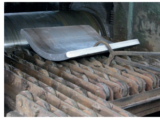
Fig. 7. Ingot widened after the cross-rolling
