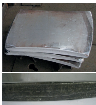
Fig. 13. Ingots of AA2519 alloy widened to ~ 600mm and prepared for rolling and cladding with EN AW-1050A alloy (single-side cladding)
