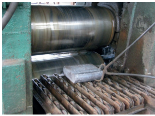
Fig. 6. The first pass of AA2519 alloy ingot through a rolling mill
