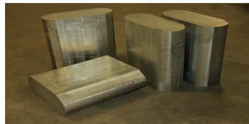
Fig. 2. Blocks prepared for the rolling process
