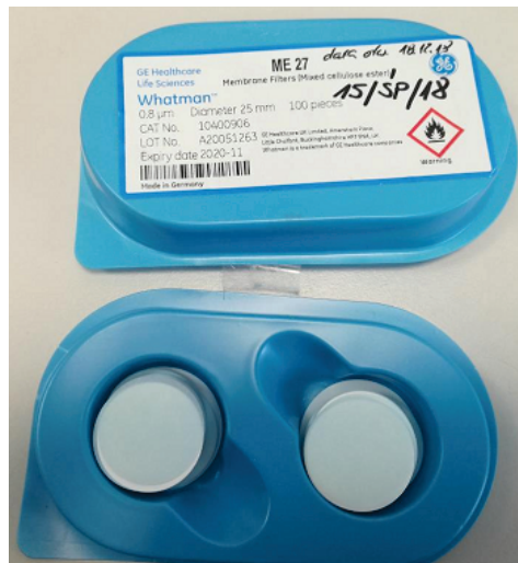
Fig. 2. An example of a membrane filter of cellulose esters of the diameter \text{Ø}25 mm intended for testing the inhaled fraction (photo K. Pikulik)
