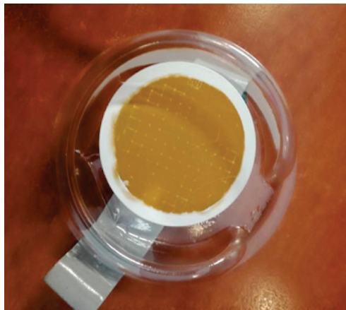
Fig. 1. An example of a filter of the diameter \text{Ø}37 mm intended for testing the respirable fraction (photo K. Pikulik)
