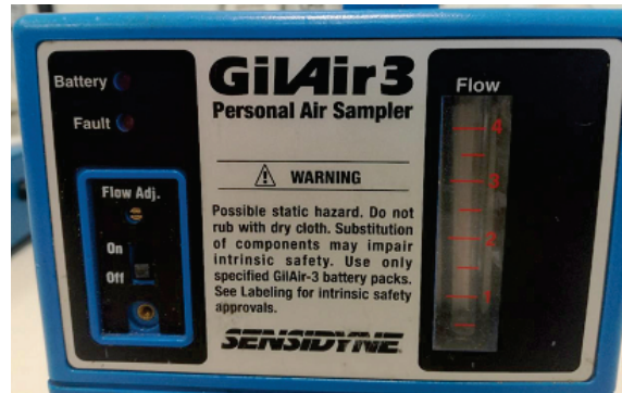
Fig. 4. Individual aspirator, type GILIAN GilAir3, applied in these tests (photo K. Pikulik)
