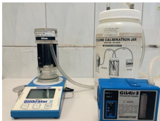
Fig. 3. A set for checking the flow of air in the aspirator together with the aspirator type GilAir3 (photo K. Pikulik)
