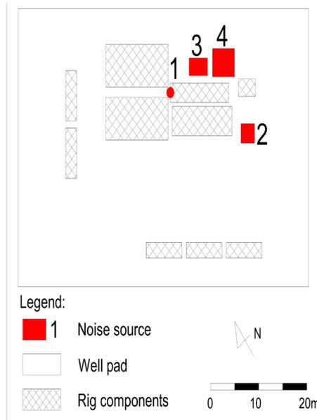
**Fig. 3.** Major sources of noise during the realization of the gas well Wieczorek-AGH-1 (1 – driving head, 2 – mud pump EMSCO HTF 500, 3 – air compressor Atlas Copco XRVS336, 4 – air compressor Atlas Copco XRRO667)
