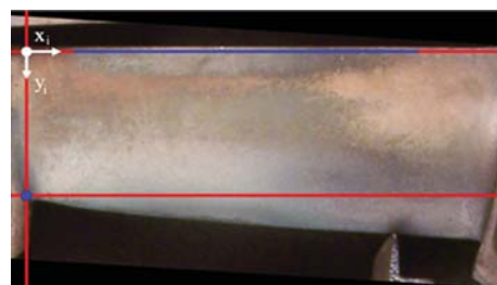
Fig. 7. Lines limiting the vane surfaces – sought (rectangular) area for further colour analysis
