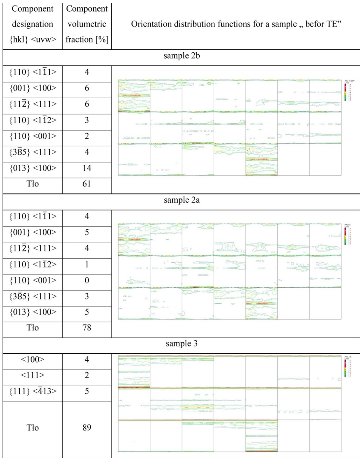
Fig. 26. The volume fraction of the main texture components in the tested samples and the orientation distribution functions
