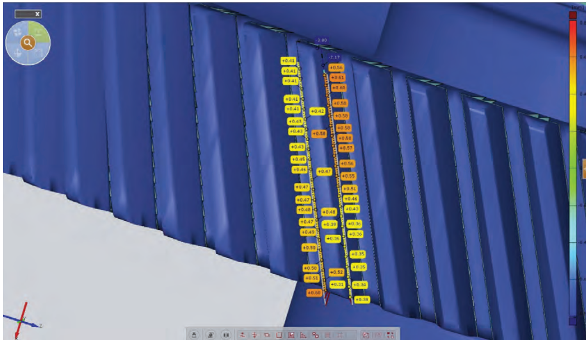
Fig. 11. The detailed analysis of tooth line deviations- position 1
