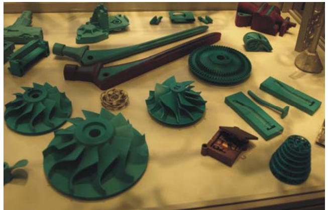
Fig. 3. Wax models made by means of Solidscape device
