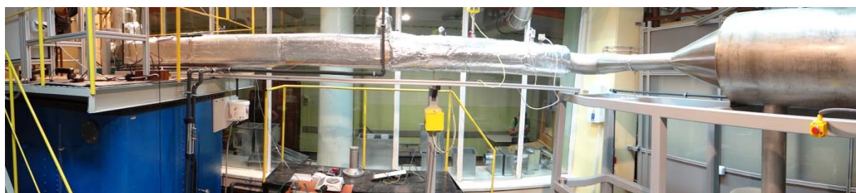
Fig. 6. Laboratory scale heat condensing exchanger with equipment (from right – flue gas generator, heat exchanger, cooling water tank)
