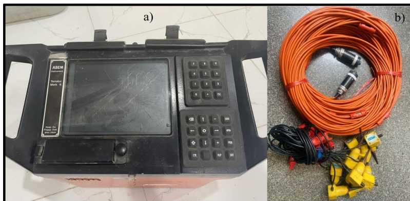
Fig. 8. Seismic equipment: a) Terraloc Mark-6 seismic probe, b) Geophones and connecting cable
