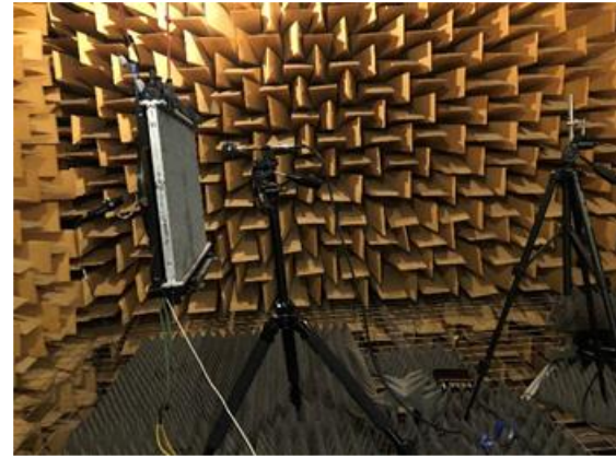
Fig. 4a. Device under test resiliently suspended in an anechoic chamber
