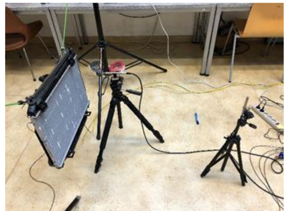
Fig. 4b. Device under test resiliently suspended in a reverberation field
