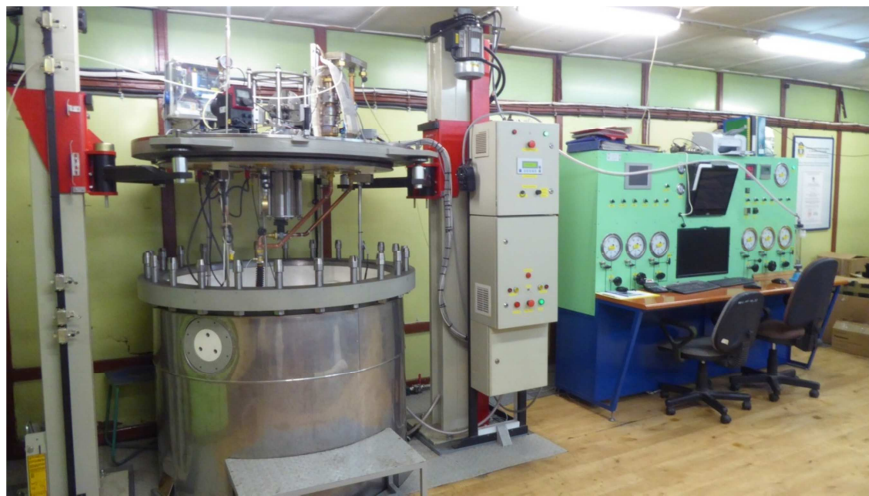
Fig. 2 Combined simulator station: respiratory, metabolic and hyperbaric.
