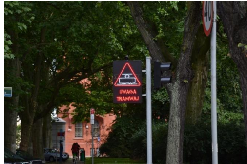
Fig. 10. A warning board with the picture of a tramway that lights up as the tram approaches – 3 Maja street in Szczecin, Poland – ‘Beware of tramway’ [Source: Młodystach 2021]
