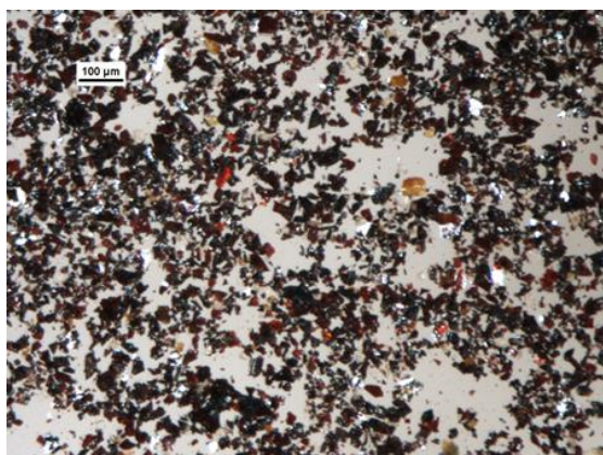
Fig. 8. Picture of the pulsating high gradient magnetic separator concentrate produced at 0.6 T
