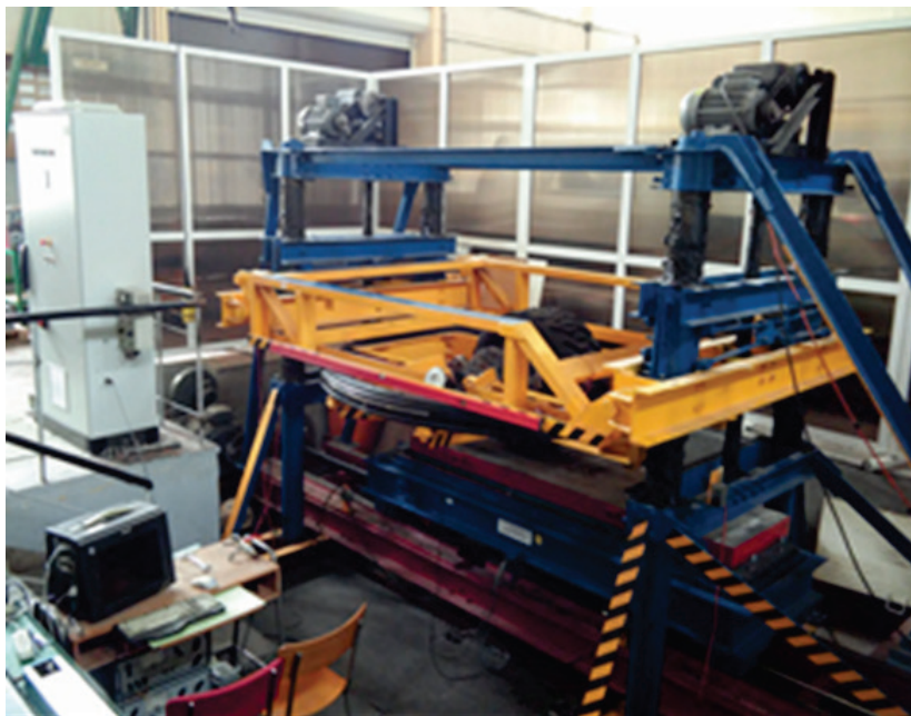
Fig. 7. The universal quasi-static indoor tire test facility
