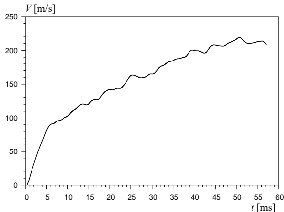
Fig. 13. Velocity of the counterprojectile as a function of time
