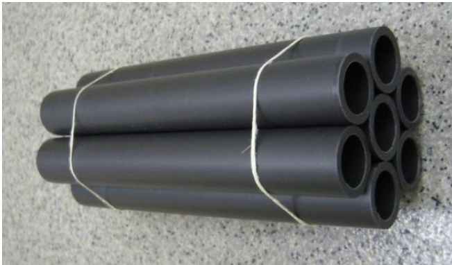
Fig. 4. Seven single grain Bazalt 2a propellant charges
