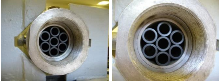
Fig. 5. Propellant charge grains inside the combustion chamber
