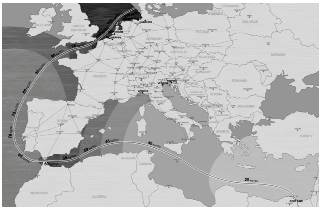
Fig. 5. Emissions of CO 2 (kg/ TEU) from vessels in maritime transport around Europe – increasing from Port Said, Egypt [6].
