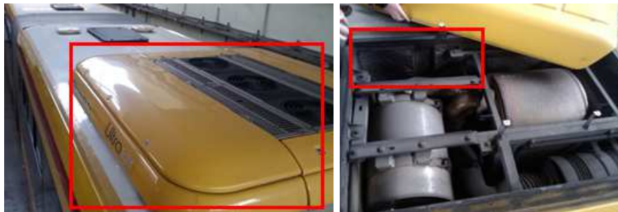
Figure 6: Preliminary ORC system location.
