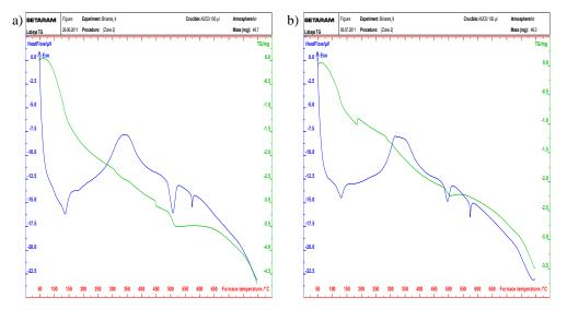
Fig. 1. Spectra DTA of concrete stencil, curves of TGA and DSC: a) reference template, b) modified template
