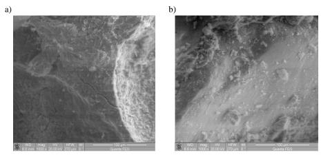
Fig. 3. Microstructure of decorative fine-grained concrete templates (X20000): a) reference template, b) modified template
