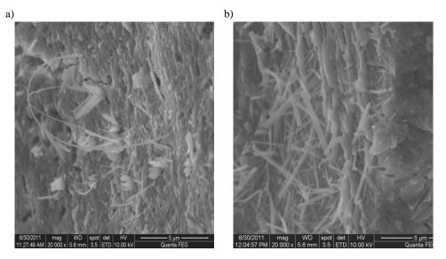
Fig. 2. Microstructure of concrete stone (X20000): a) reference template, b) modified template
