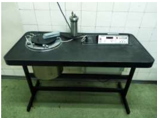
Fig. 2. Test stand with calorimeter
