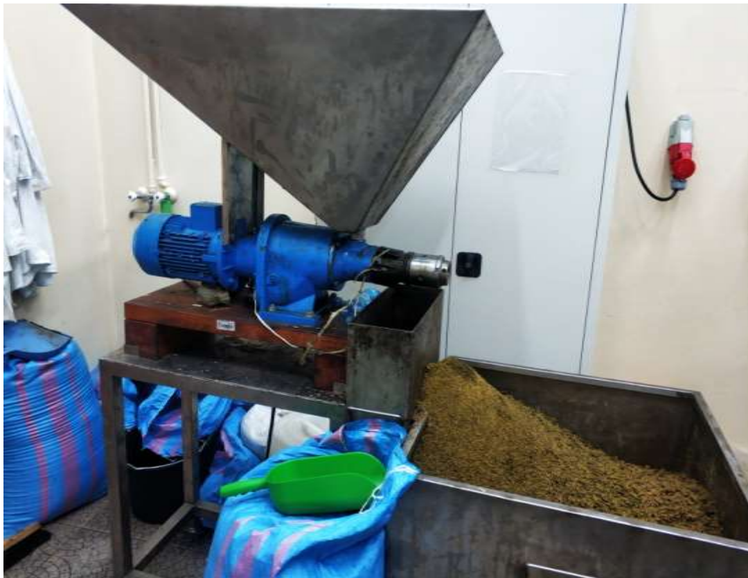
Fig. 1. Test stand with the UNO press made by FARMET
