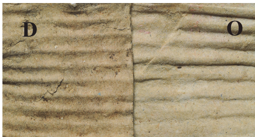
Fig. 2. Fibres of a PB samples, after 1-month experiment in sandy soil
