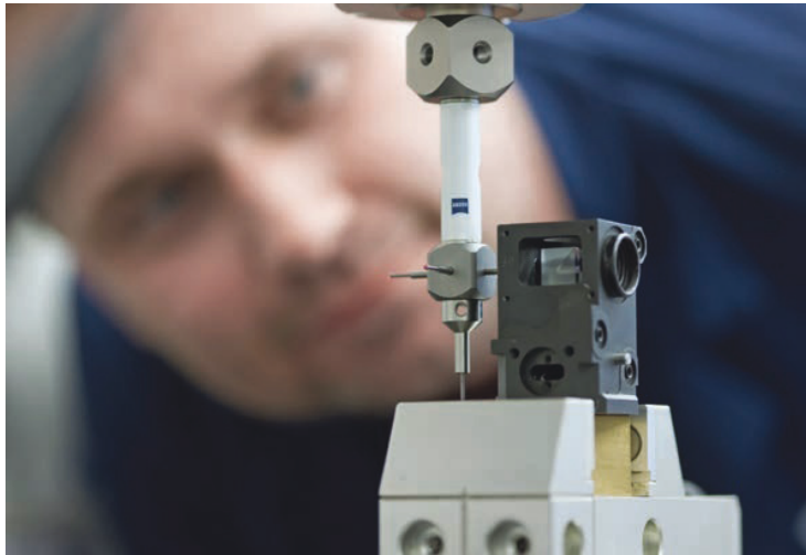
Fig. 7. FISBA Optik uses the ZEISS MICURA to also measure mechanical parts and prototypes with the utmost accuracy
