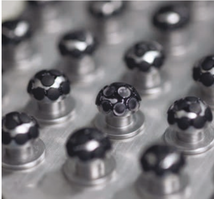
Fig. 5. In order to grind the lens elements, they must first be mounted with pitch
