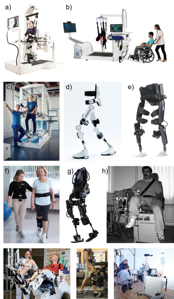
Figure 2. Contemporary rehabilitation robotic systems for lower extremities – a) Lokomat [10], b) ReoAmbulator [15], c) G-EO [16], d) HAL [7], e) ReWalk Personal 6.0 [18], f) ReStore [18], g) EksoNR [5], h) MotionMaker [9], i) Anklebot [20], j) PHYSIOTHERABOT [42], k) RENU-1 [14]
