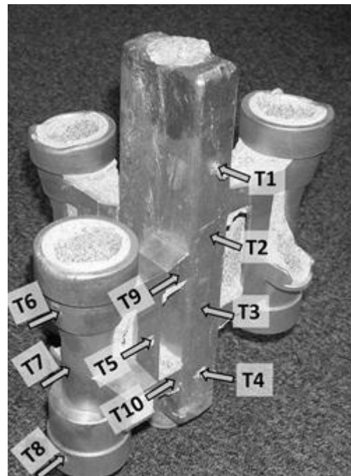
Fig. 2. Thermo elements location scheme in the ceramic mold regarding the casting
