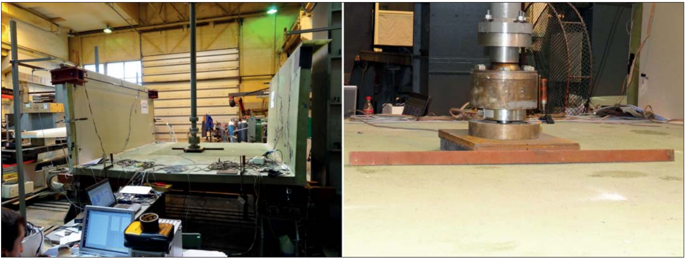
Fig. 5. Force applied at the middle of platform's width and length
