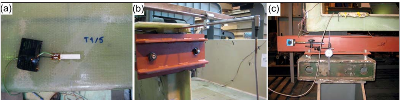
Fig. 6. Sensors used during experiment: (a) strain gauge, (b) displacement sensor, (c) dial gauge with rubber bearing
