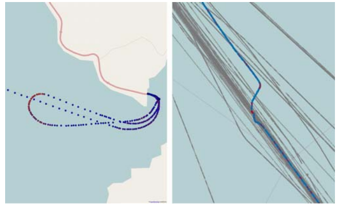
Figure 6: LEFT - Position trace of a RO-RO vessel, color coded according to the ROT (high ROT - red, low ROT - blue), imposed on a map. A sharp turnaround, with a high ROT is visible, which most probably is not an emergency situation. Taking the time (8th May, 21:53) and the following short stay in port (~ 3 minutes) into account, it rather indicates that the vessel was empty and had a late customer pick up. RIGHT - Regular tracks of a ferry in gray (over half a year), indicate that the normal path is straight ahead. An unusual maneuver, as detected by our algorithm (color coded according to the ROT) is also shown. This may indicate that an obstacle (non-AIS emitting object, e.g. fishing net) was encountered, causing correction of course compared to the normal behavior.
