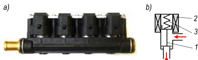
Fig. 1. STAG AC W02 – four-section injection rail LPG/CNG: a – picture; b – scheme: 1 – plunger, 2 – electromagnetic circuit, 3 – spring, red arrows point at the flow direction
