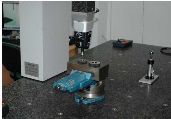
Fig. 2. The experiment setup. Zeiss WMM850S equipped with Renishaw PH20 probing system and reference rings
