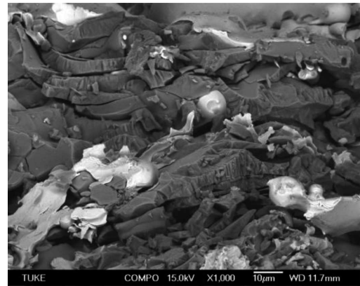
Fig. 9. Al 2 O 3 coating sandwich structure on the fracture area
