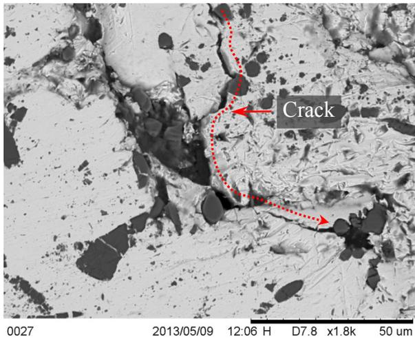
Fig.3. Microstructure of composite material Cu-10 vol.% Saffil after bending in fractured region with propagation of crack thorough Cu matrix between  $Al_2O_3$  fibres.
