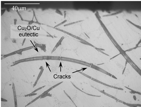
Fig.2. Microstructure of Cu-10 vol.% Saffil fibres composite materials examined at 300°C with fragmented fibres subjected to tension stresses.
