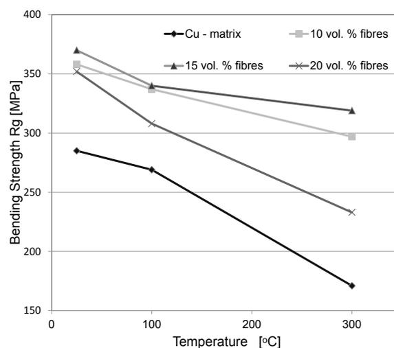
Fig. 6. Bending strength of unreinforced and copper based composite materials strengthened with 10, 15 and 20% of alumina fibers.
