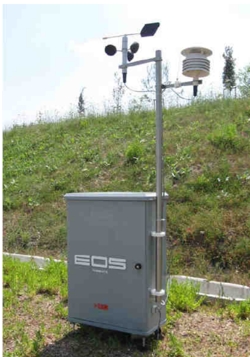
Fig. 4. Electronic nose EOS 507 used for terrain measurements [26]
