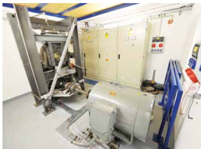
Fig. 3. Tram wheel stand with PMSM drive; photo: ERCT [2]
