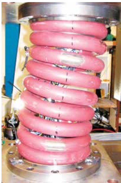
Fig. 6. Testing of a secondary flexi-coil spring on the dynamic test stand
