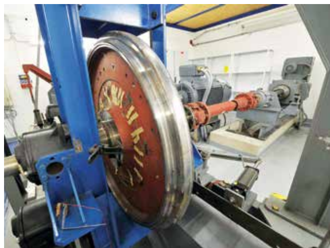
Fig. 2. Wheel/rail test stand in the ERCT; photo: ERCT [2]
