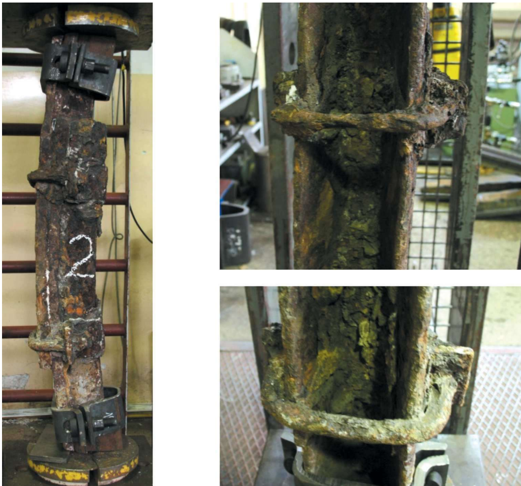
Fig. 4. Friction joint 2 prepared for testing and shackle technical condition
