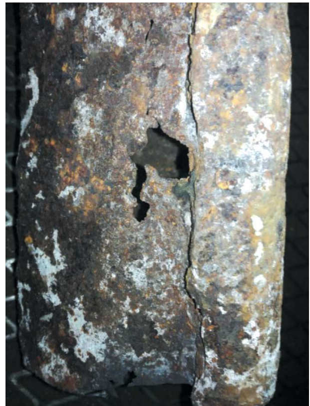
Fig. 2. Section perforation in flange area
