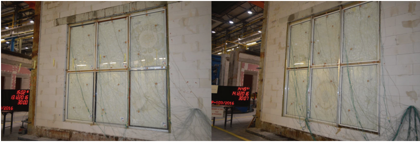
Fig. 5. The view of the unexposed surface of tested specimen No. 1 during the fire resistance test
