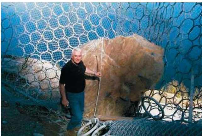
Fig. 3. Tested and certified RX-300 Rockfall Barrier after an impact, Telemark/Gvaleviken, Norway
