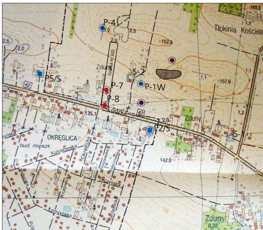
Legenda: P2/S; S-1; S-2; P5/S – studnie; P-1W; P-4 – piezometry
