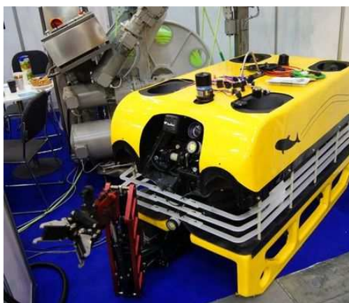
Fig. 3.6. Multi-purpose underwater vehicle "Morświn" designed at the Gdańsk University of Technology.
