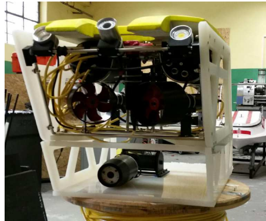
Fig. 3.14 Modular system for the exploration of aquatic environments and underwater objects built by Forkos Ltd. within the IE OP project no. 01.04.00-22-069/13 (the system comprises two cooperating underwater vehicles: miniROV KH-200 and microROV Frog).
