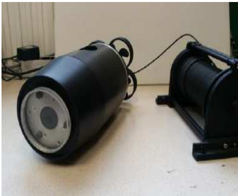
Fig. 3.15 MicroROV Frog developed by Forkos Ltd. within the IE OP project no. 01.04.00-22-069/13 with an automatic cable winch and a special TV system for dimensioning underwater objects.
