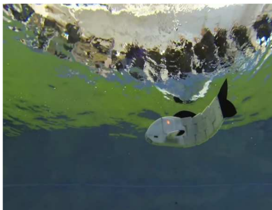
Fig. 3.10. One of the concepts of an underwater biomimetic vehicles developed within the 'Śledzik' project.
