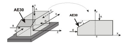
Fig. 4. An example of indicating the basic datum surface for machining located with the angle  $30^{\circ}$  in relation to A and B basic datum surface [source: own study]
