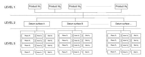
Fig. 1. Structure of database for saving data on casing-class products to be machined in a FMS [source: own study]
