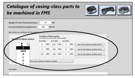
Fig. 8. The form for defining datum surfaces for machining [source: own study]
