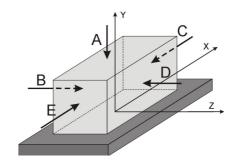
Fig. 3. Literal denotation of basic datum surface for machining [source: own study]
