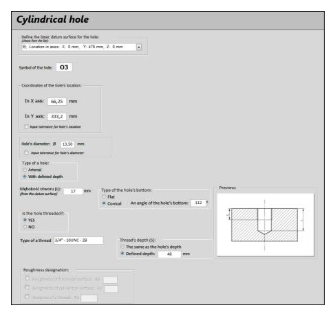
Fig. 11. The form of saving data about the object (an example of cylindrical hole) [source: own study]
