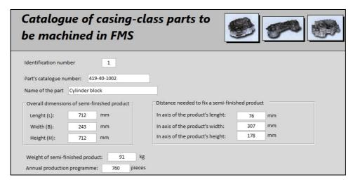
Fig. 7. Main form to input data about parts to be machined in FMS [source: own study]
