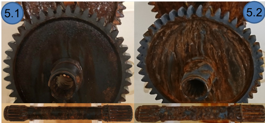
Fig. 5. The gear wheel and torsion shaft with phosphate coating after 120 h (5.1) and after 240 h (5.2) NSS test
