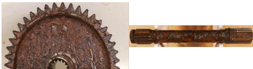
Fig. 2. The gear wheel and a torsion shaft without any galvanic coatings after 120 h NSS testing
