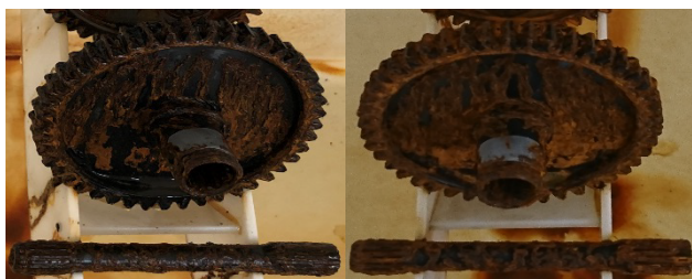
Fig. 3. Oxidized gear wheel and torsion shaft after 165 hours (left side) and after 240 hours (right) NSS test.
