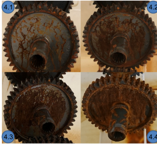
Fig. 4. The gear wheel with oxidophosphate coating after 70 h (4.1); 120 h (4.2); 165 h (4.3) and 240 h (4.4) NSS test
