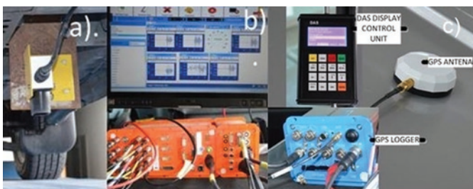
Fig. 2. Measurement equipment used to conduct the tests in real-world conditions
